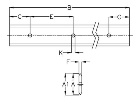
$\begin{array}{lll} A & = 76 \\ A1 & = 77.58 \\ B & = 4496 \\ C & = 43.0 \\ E & = 90 \\ F & = 9.43 \\ For bearing = J54 \end{array}$
